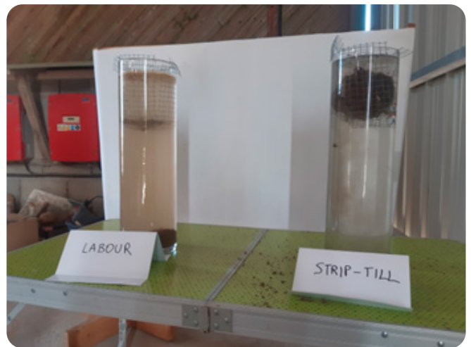
Effect of water action on ploughed soil (on the left) and no tilled soil (on the right).
