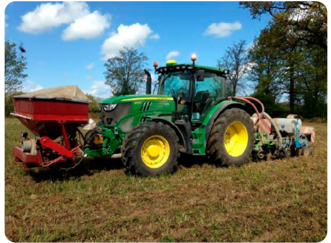
Strip-tiller equipped with frontal fertilizer tank and combined to maize seeder.
