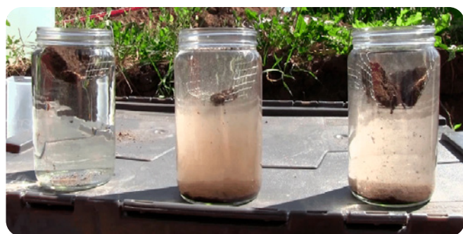
Simple aggregate stability test of soil in water using a coarse metal mesh
