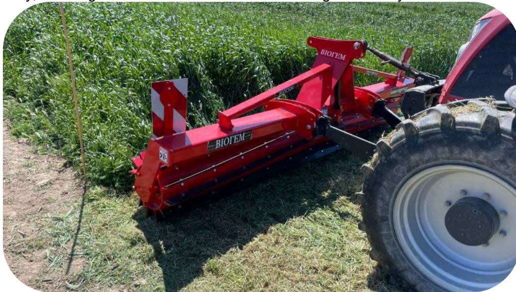
Figure: Mechanical termination of a triticale cover crop with a roller-crimper, Source: C. Vasilikiotis-Perrotis College, 2023
