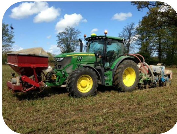
Figure: Strip-tiller equipped with frontal fertilizer tank and combined to maize seeder. Source: Gabriele Fortino
