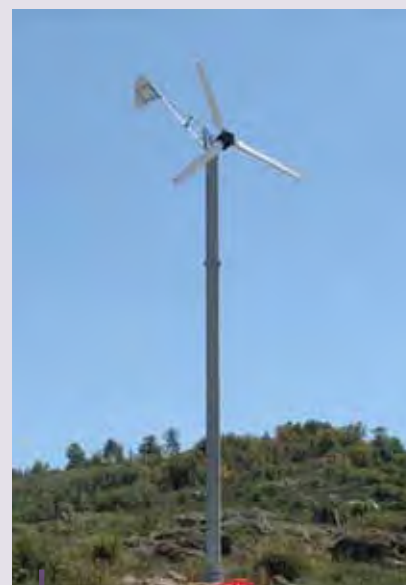
Micro wind turbines generate electricity. Their light weight, small size, and flexible configuration allows them to be installed in both urban and rural environments.
