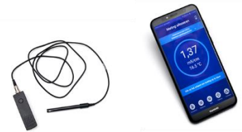
The AquaMobile (handheld device to measure EC in surface waters) developed in this project
