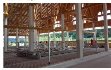
In the production part there are 130 sleeping stalls. The new cowshed also accommodates 20 sleeping stalls for the cows in dry period. 4 x 15 m space is used for the nursery using deep litter housing system. Cow neck shackles are made of glass fiber and not of metal as it is most common.
